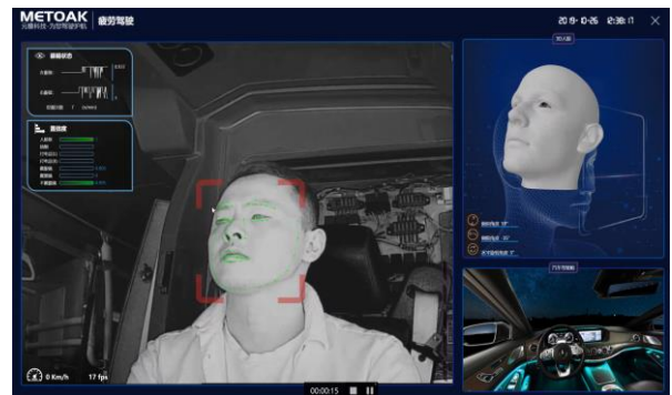
Figure 5. The Driving Drowsiness Detection System (DDDS)
