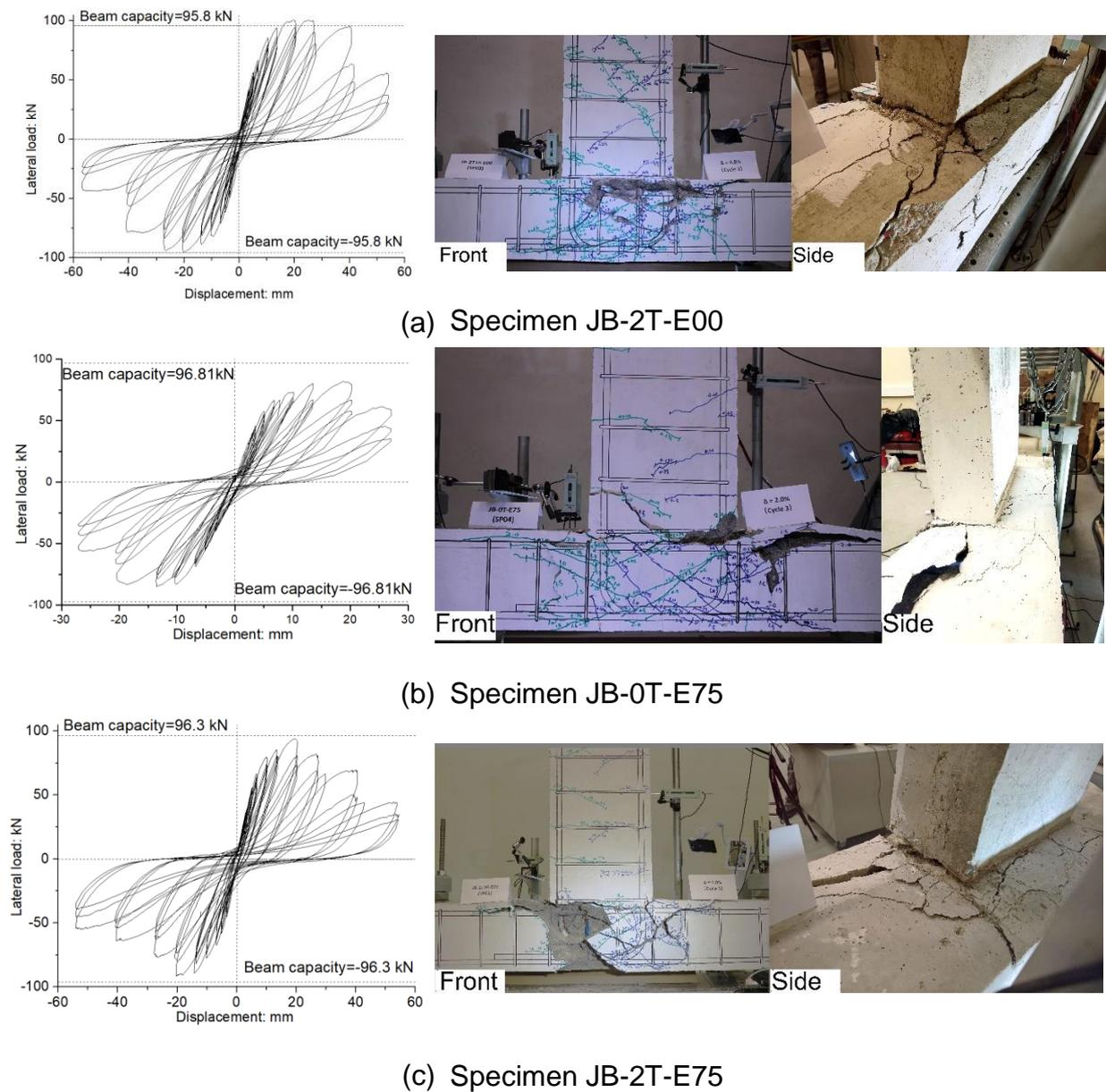
Fig. 4 Hysteretic covers and the cracks patterns
