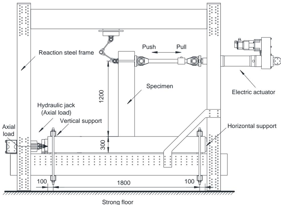
Fig. 2 Test set-up
