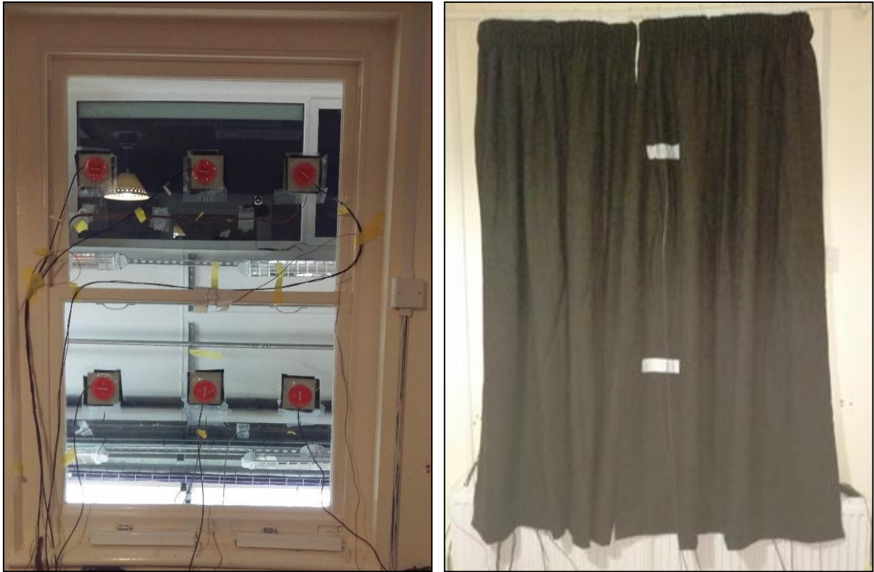
Figure 3: U-value measurement setup showing positions of heat flux sensors (left) and with tweed curtain (right)
