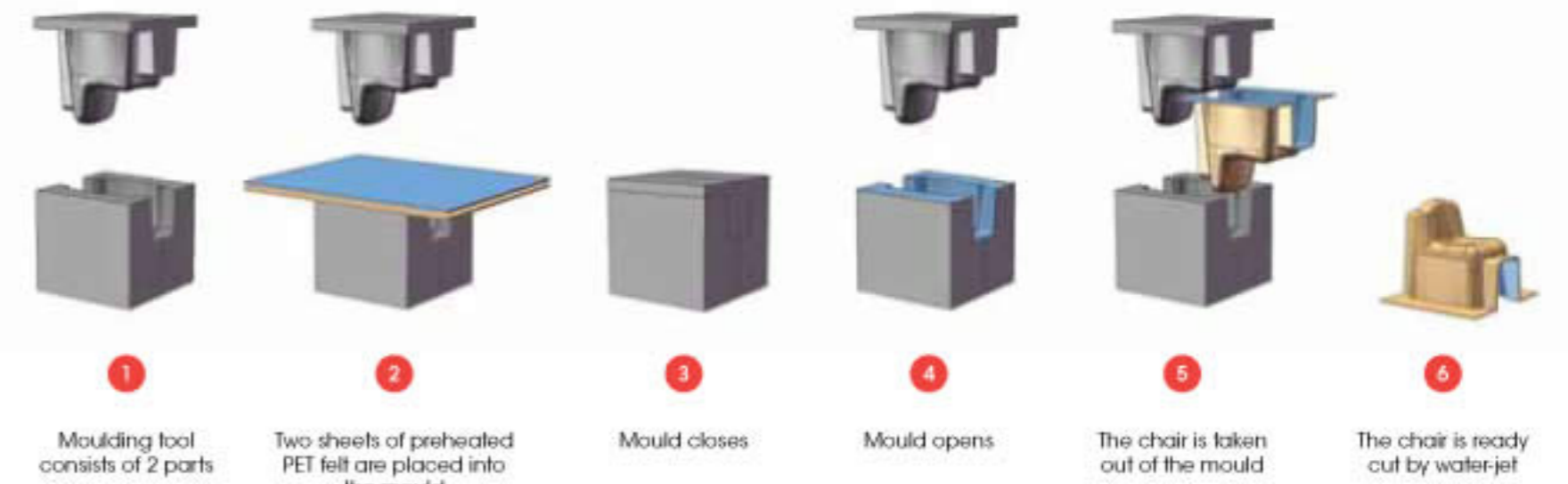
BELLOW THE MOULDING PROCESS OF THE NOBODY CHAIR
