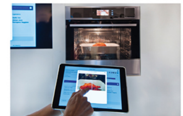
Top: A modern kitchen unit in EuroCucina. Above: an in-cooker camera viewed remotely on an iPad
